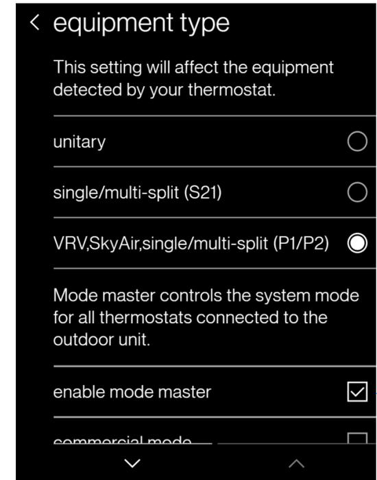
**Note: Releasing the changeover master by uncheck “enable mode master”**
