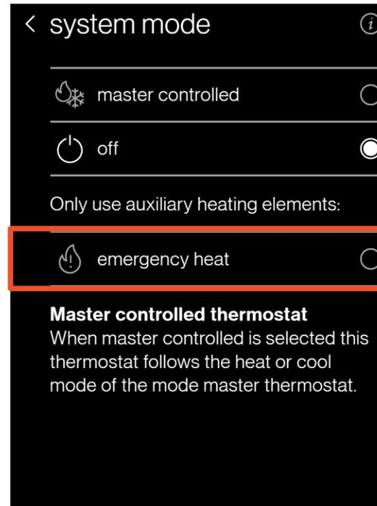
**Note:** The Emergency Heat mode will engage the AUX heater contact ONLY, however the IDU and the Fan will be OFF.
