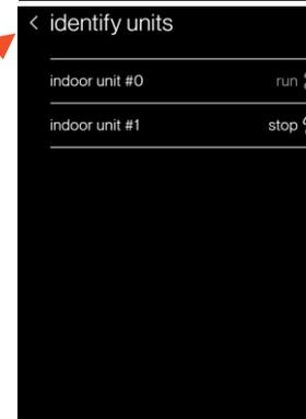
Identify the indoor unit by force fan on
