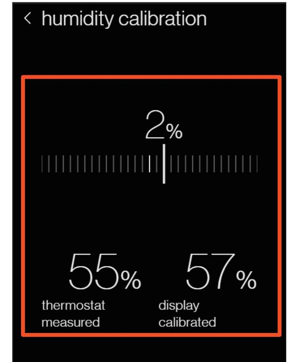
Note: The system needs to be in the “off” mode during the calibration
