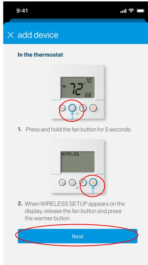
2. Press and hold the fan button on the thermostat for 5 seconds to put the thermostat in "Wireless Setup" mode. Then press the up/warmer button on the thermostat to display the 6-digit pairing code and select "Next".
