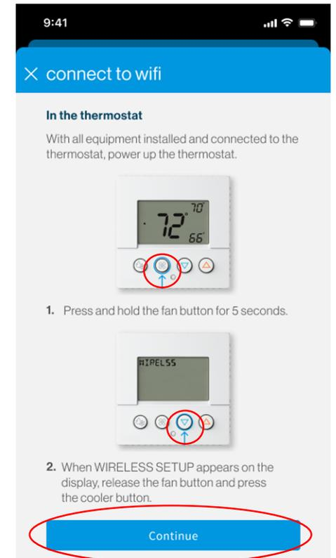
4. Press the fan button for 5 seconds, then press the cooler/down button to put the thermostat in “AP MODE”, then select “Continue”.
