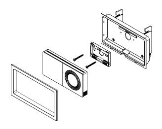
Face plate Thermostat Screws Terminal plate Flushmount
