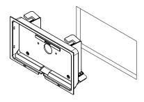
Tighten screws to align mounting tabs.
